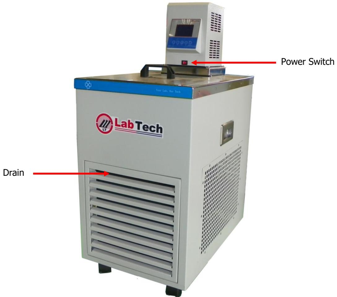
**NOTE: the drain outlet is in the middle position inside the front air grid. Turn the thread stem beside it to drain the liquid out.**
