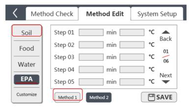
c) Step 01: Touch the Temp. Text box, input 100 via the digital key. Then touch Time text box to input -2 which means heat in max. heating speed (Normally, the average heating speed is around 5°C/min).
