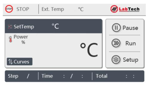
LabTech iTouch controller operates by simply touching the keys on the screen. Connect the iTouch controller to the back of DigiBlock main unit, switch ON the DigiBlock and the iTouch screen is automatically ready for operations.
